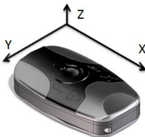
Figure 13 Accelerometer axis directions
